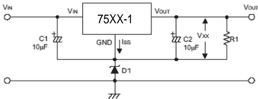
$$V_{OUT} = V_{XX} + VD1$$
