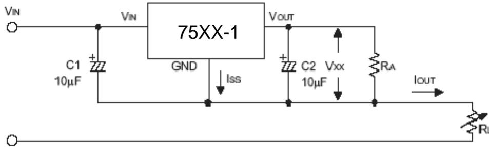
$$I_{OUT} = V_{XX}/R_X + I_{SS}$$
