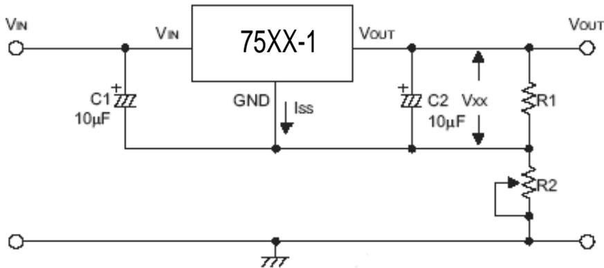
$$V_{OUT} = V_{XX} (1 + R2/R1) + I_{SS} * R2$$
